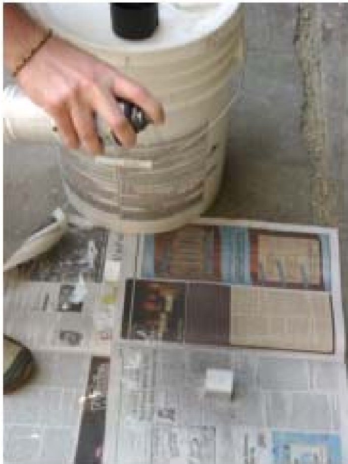
Figure 2.2: Applying speckle pattern.
