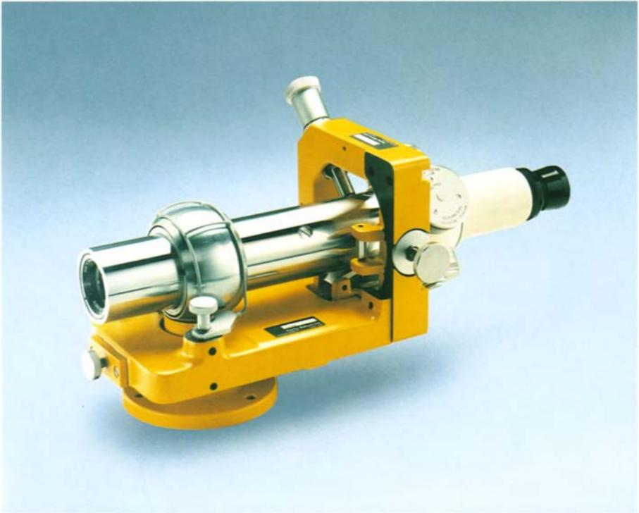
**Plate VIII** *Straightness – alignment telescope. Illustrates pivot around spherical collar (courtesy Taylor Hobson Ltd)*
