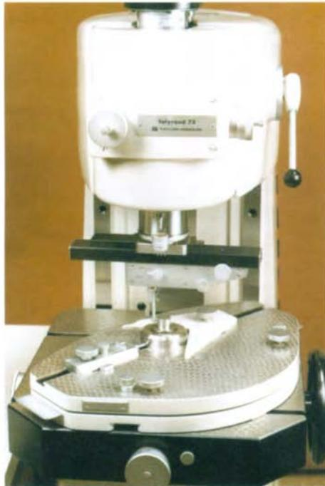
**Plate X (b)** *Internal cylinder measurement, and external illustrates workpiece positioning methods (courtesy Taylor Hobson Ltd)*
