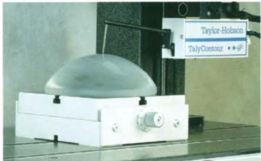
**Plate V** *TalyContour Series (a) and (b) Show calibration (c) Demonstrates wide range, high resolution (courtesy Taylor Hobson Ltd)*
