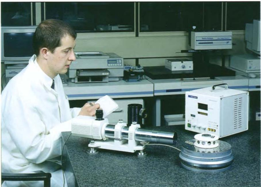
**Plate IX (b)** DA20 Autocollimator with reference index table used to calibrate a polygon (courtesy Taylor Hobson Ltd)
