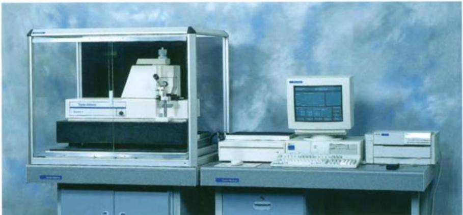
**Plate VII** *The Nanostep, successor to Talystep, illustrates environmental insulation (courtesy Taylor Hobson Ltd)*
