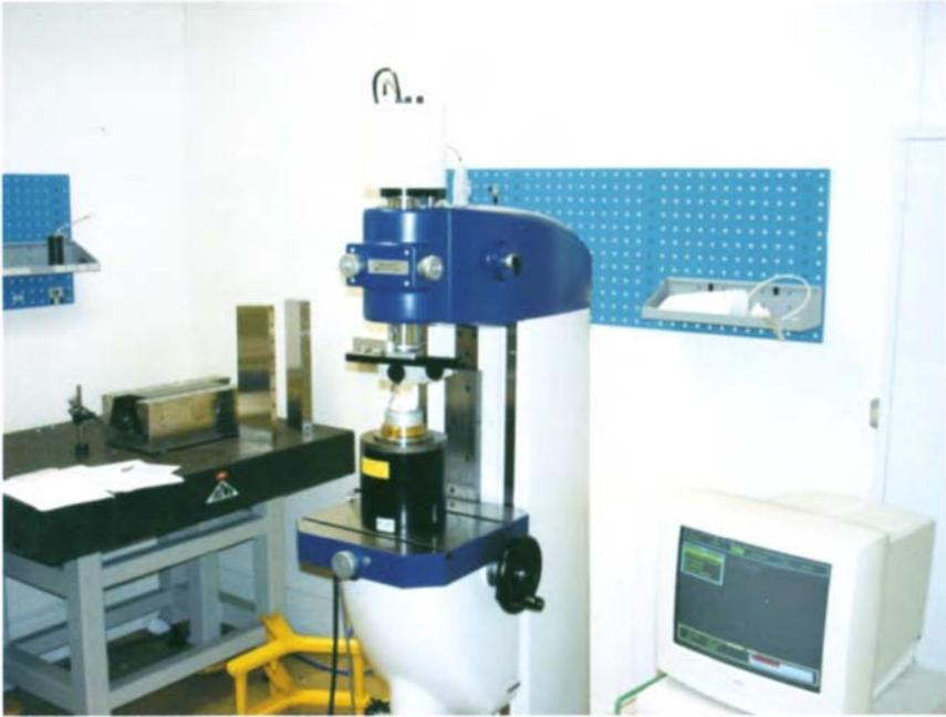
**Plate XVI** *Set-up apparatus – roundness calibration (courtesy Taylor Hobson Ltd)*
