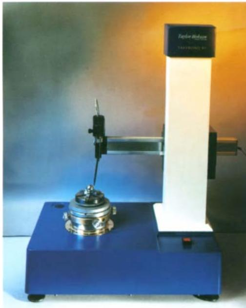
**Plate XV** *Talyrond 31 – cylindricity measurement (courtesy Taylor Hobson Ltd)*
