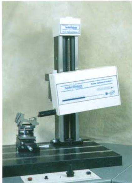
**Plate IV** P.G.I. Integrated instrument (a) Interchangeable stylus (b) Wide range (c) Versatile positioning (courtesy Taylor Hobson Ltd)
