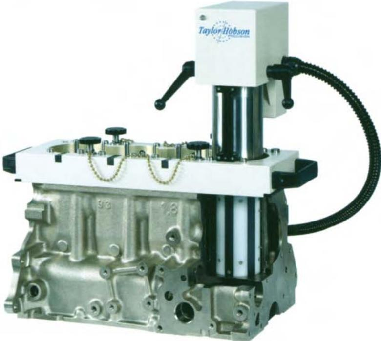
**Plate XI** *Portable rotating pick-up roundness measurement shows the measurement of cylinder bores (courtesy Taylor Hobson Ltd)*
