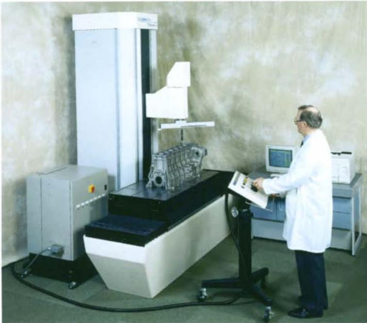
**Plate XII** Large rotating spindle roundness instruments (courtesy Taylor Hobson Ltd)
