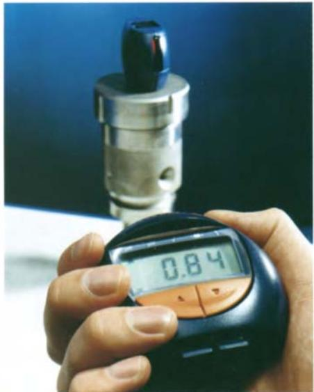
**Plate II** (a) Hand-held instrument (b) Sutronic Duo instrument measuring surface of cylinder head and piston (c) Remote operation – numerical output (d) Remote operation (courtesy Taylor Hobson Ltd)
