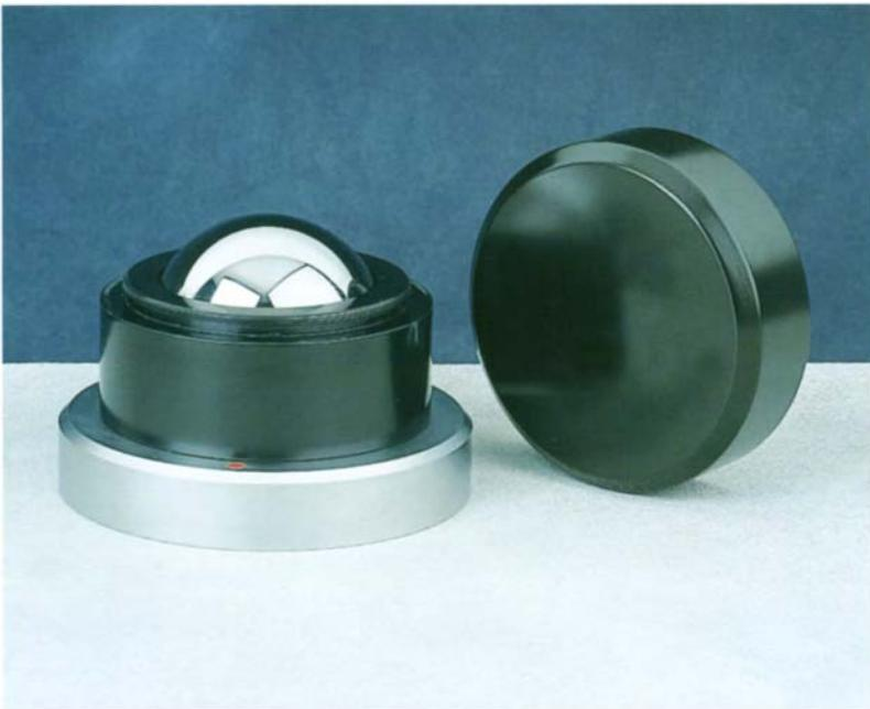
**Plate XVII** *Calibration and curvature artifact (courtesy Taylor Hobson Ltd)*
