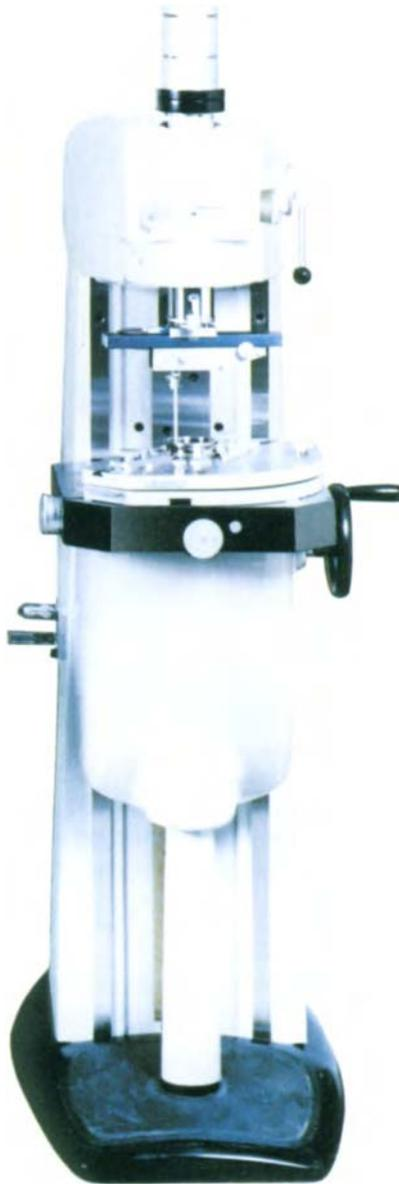
**Plate X (a)** *A rotating spindle instrument Talyrond 73. The ultimate in rotational accuracy (courtesy Taylor Hobson Ltd)*
